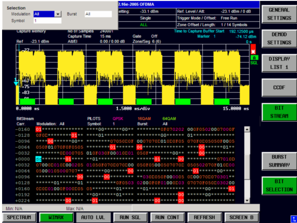
Fig. 30 Bit-Stream for OFDMA, showing the Bit Selection dialog and highlighted pilot errors.
