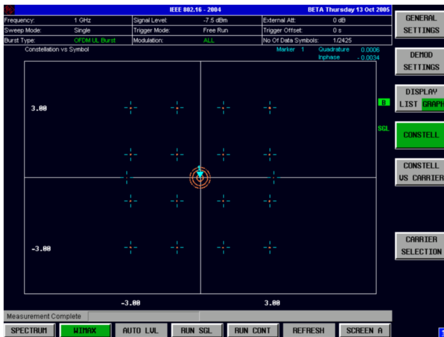
Fig. 71 IQ imbalance influence on the unallocated carriers using subchannel index 4
